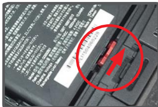
Move the slider to the right to unlock the battery.
