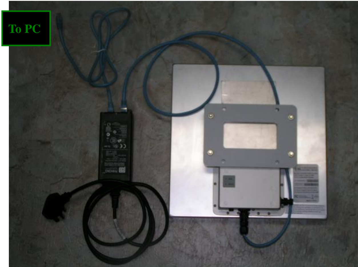
Figure 4-6 POE adaptor Setup
