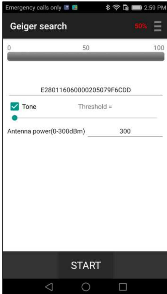
Press Start. Continuous reading will begin showing the RSSI, as well as, a beeping a tone if the Tone box is selected. The Threshold can be adjusted to limit the tone.
