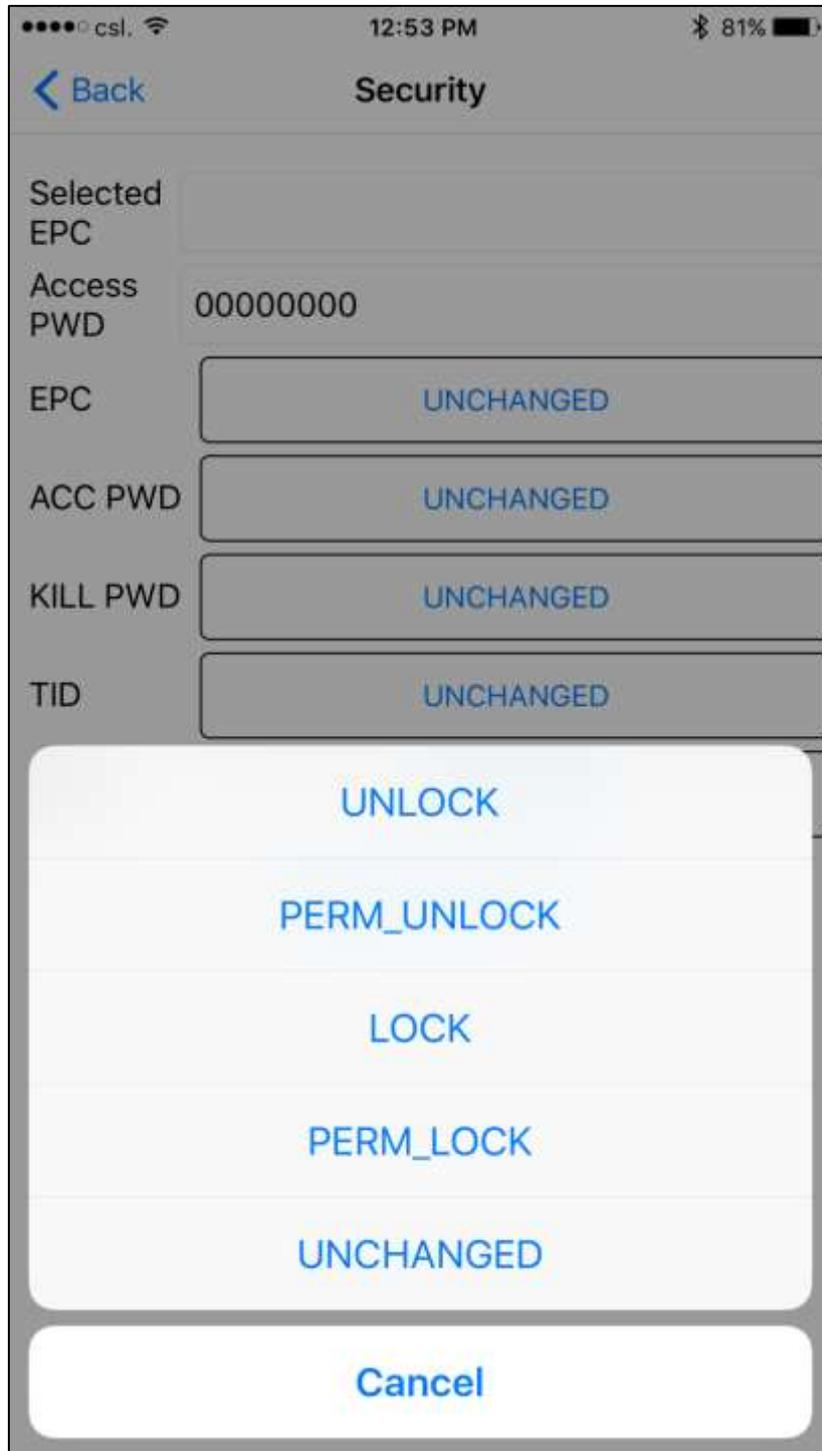
You can lock, unlock, permanently lock, and permanently unlock a memory bank of the tag. The detailed definitions of these 4 operations can be found in the EPC Global document which can be found on the EPC Global website:
