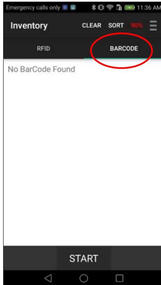
Press the START button on the touch screen or Pull the Trigger. The red LED of the barcode reader will light to help you aim the CS108 barcode scanner to the barcode. A focused circular aiming dot will appear. This indicates the optimal reading distance between the CS108 and the barcode.
