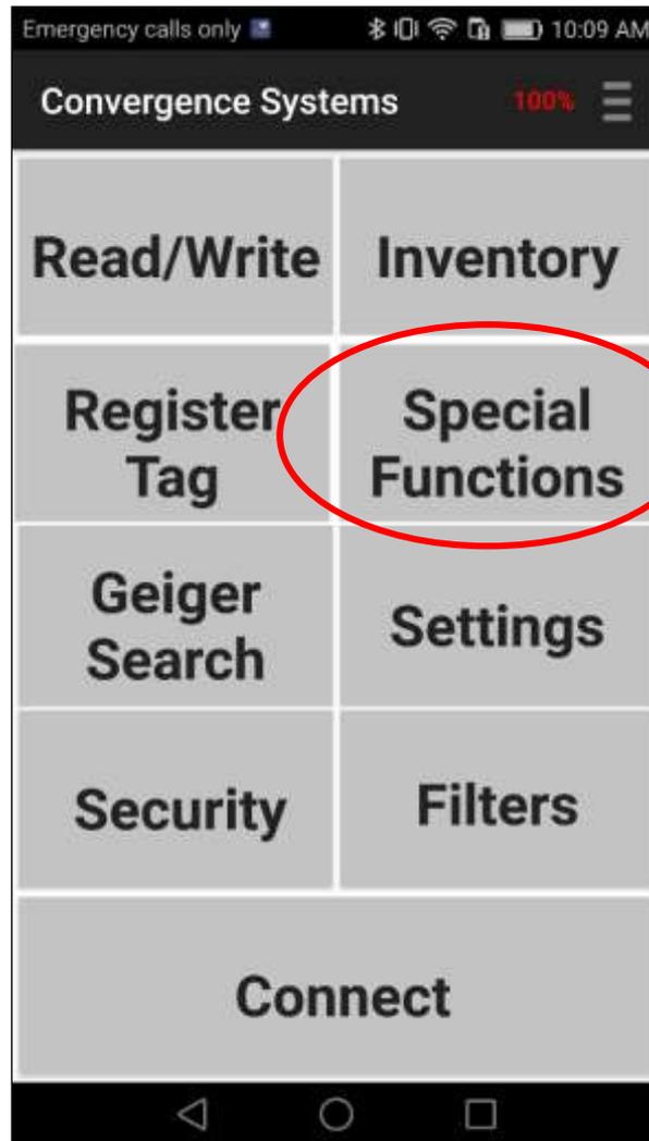
Multibank inventory is a special function that allows the RFID inventory of multiple tag memory banks at the same time.
