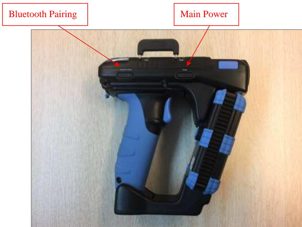
**Figure 4-3 CS108 Reader Right Side View**
