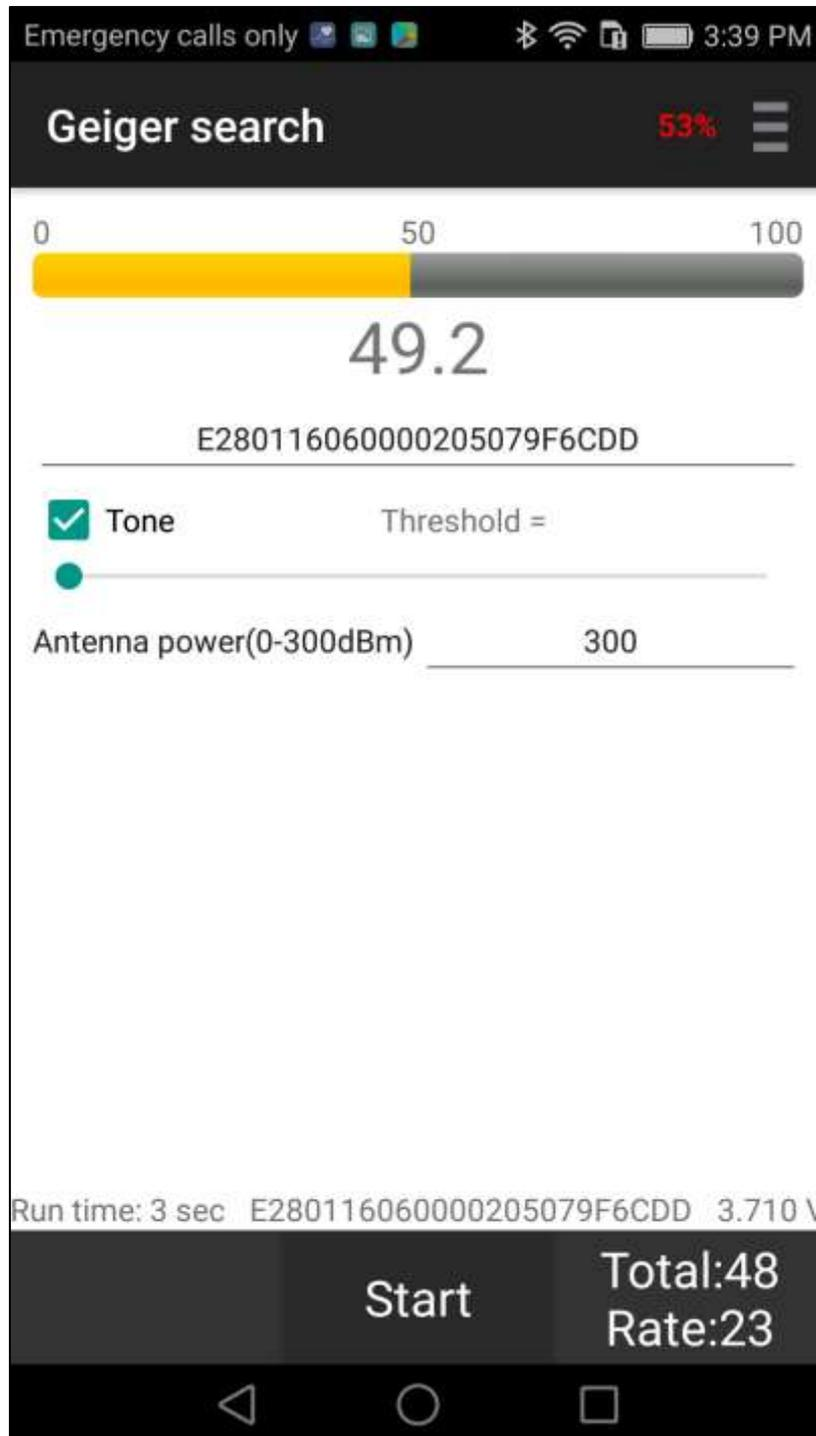
The tag can now be searched for using the beeping sound. If the Tone box is enabled, it will become faster and faster as the RSSI increases. When you are really close to the tag a long beep will replace the tone.
