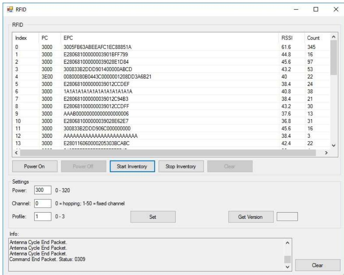
Figure 5-1 PC Application Screen – controlling CS108 via USB
