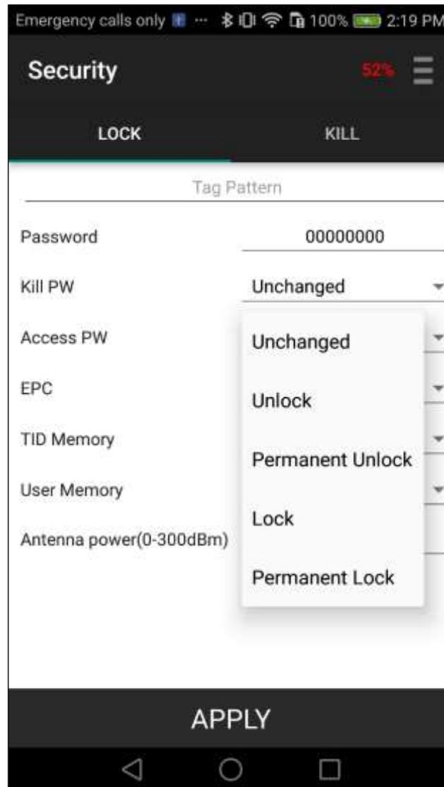
You can lock, unlock, permanently lock, and permanently unlock a memory bank of the tag. The detailed definitions of these 4 operations can be found in the EPC Global standards document which can be found at the EPC Global website:
