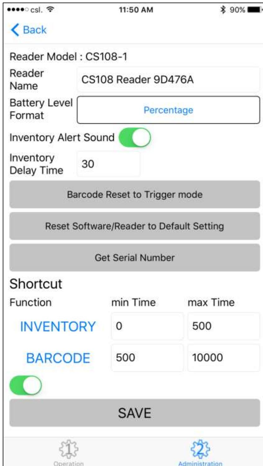
1. Reader Model is the model of the reader, for example, CS108-1 for 865-868 MHz band or CS108-2 for 902-928MHz
