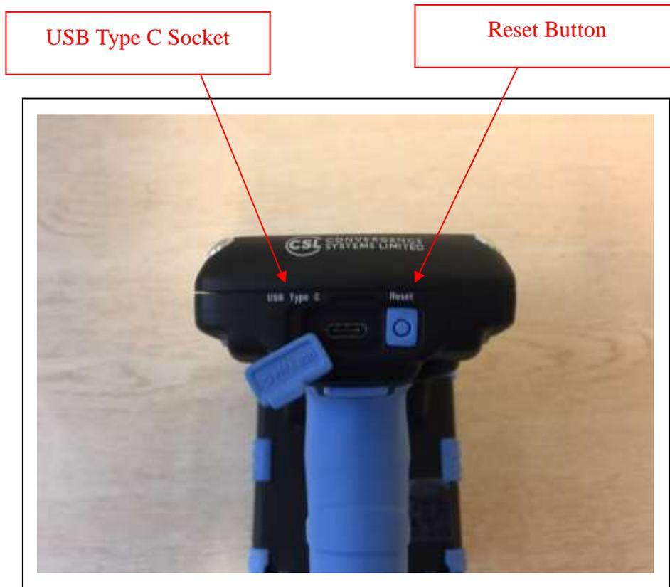
**Figure 4-4 CS108 Reader Rear Side View**
