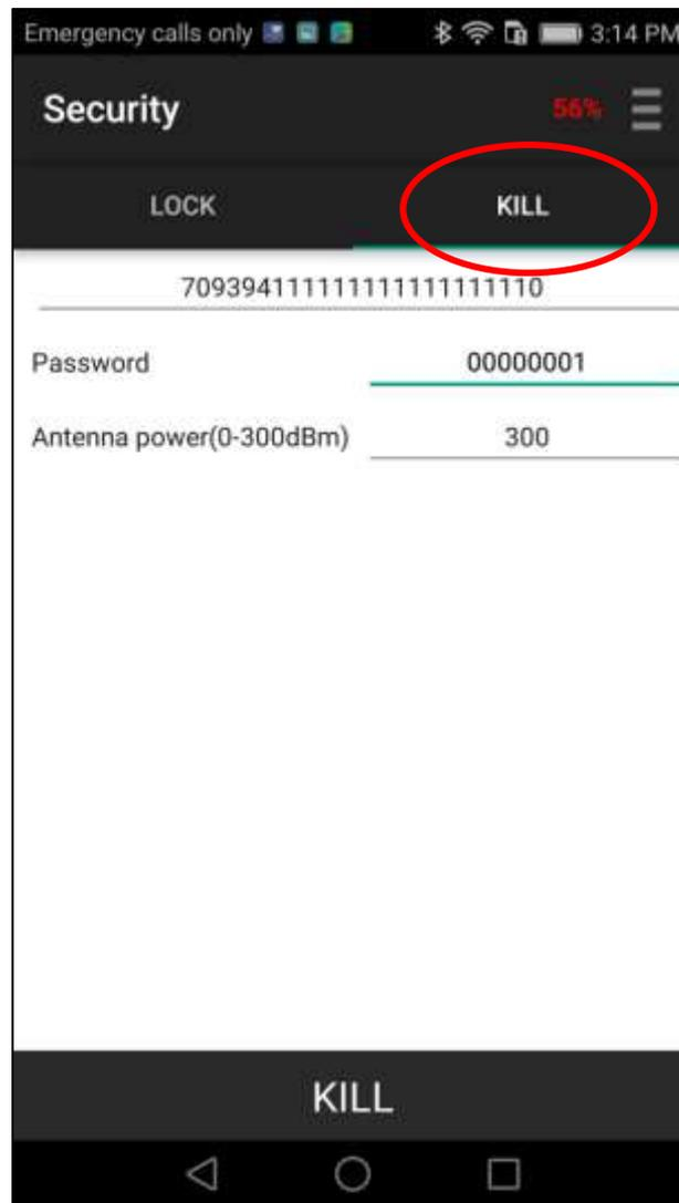
After entering the correct password, press KILL button at the bottom of the screen, the tag will be killed. During the process, the word “KILL” will be changed to “KILLING”, and, if successful, a “Success” message will pop up above the bar.
