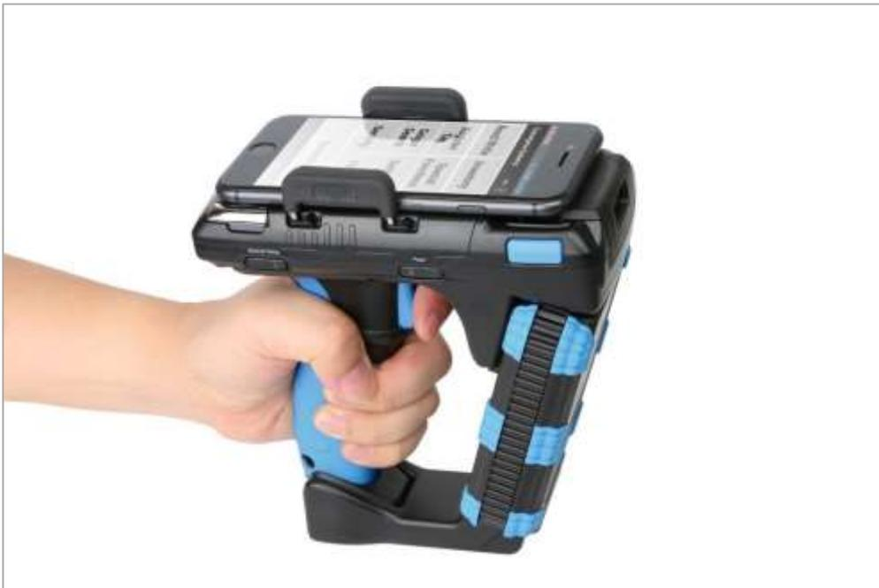
**Note:** The Smart phone App directly searches and pairs with CS108. There is no need to first pair with the CS108 via the normal Bluetooth Device connection page of the OS. Therefore, install the App on your smart device first and then search and connect the CS108 from inside the App.
