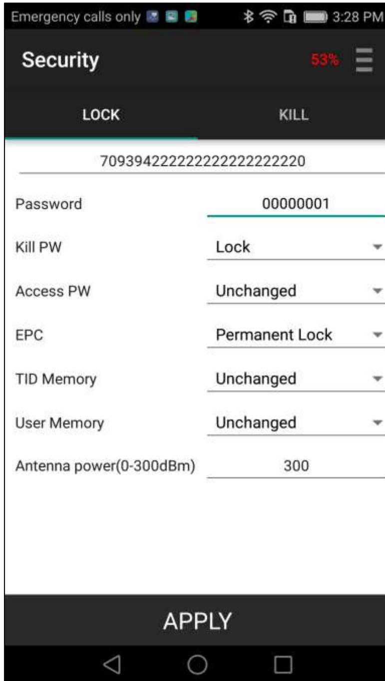
Reminder: The Lock password must be non-zero for you to be able to implement any security action. This is an EPC Global Standards definition and requirement.
