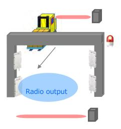
③ The forklift passes the exit sensor. The radio wave output stops. The revolving light turns off.
