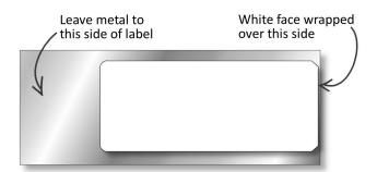
Smallest recommended bending diameter of the Confidex Steelwave Flex<sup>™</sup> is 50mm. For optimal read range please bend the label in the orientation shown below. Note that with smaller assets it is recommended to bend the label to other direction for optimal adhesion.
