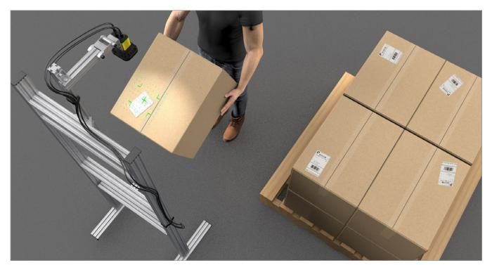
Build pallets faster by deploying overhead hands-free barcode reading stations
