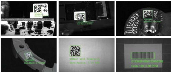
1DMax with Hotbars technology deliver high-speed reading of damaged or poorly printed 1-D barcodes as small as 0.8 pixels per module (ppm).
