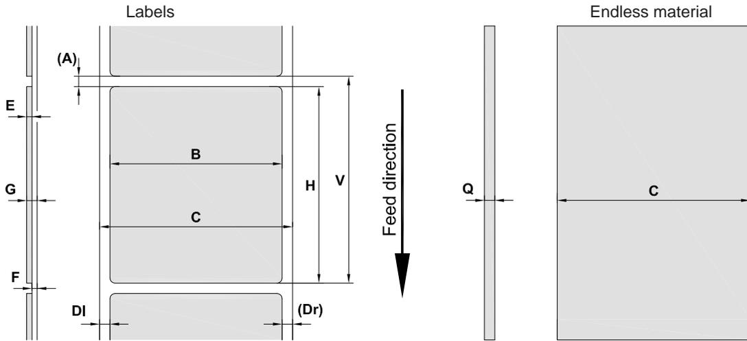
Fig. 18 Label / endless material dimensions
