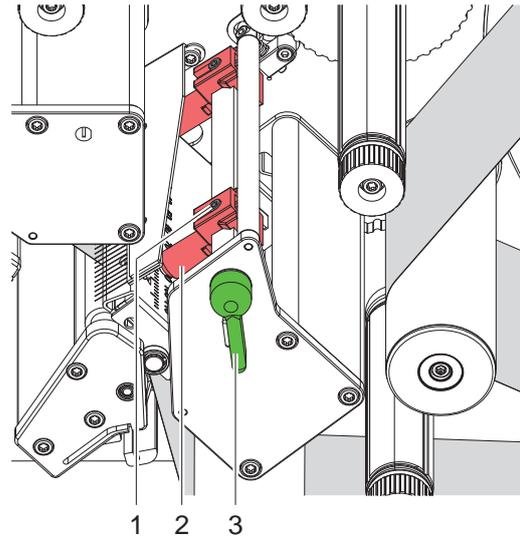
Fig. 13 Setting the lower head locking system
