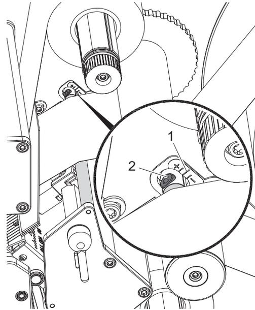
Fig. 17 Setting the lower ribbon feed path
