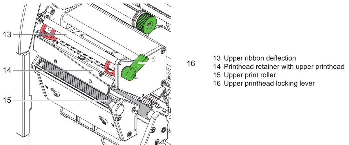
Fig. 2 Print mechanics - upper print unit for printing the main color
