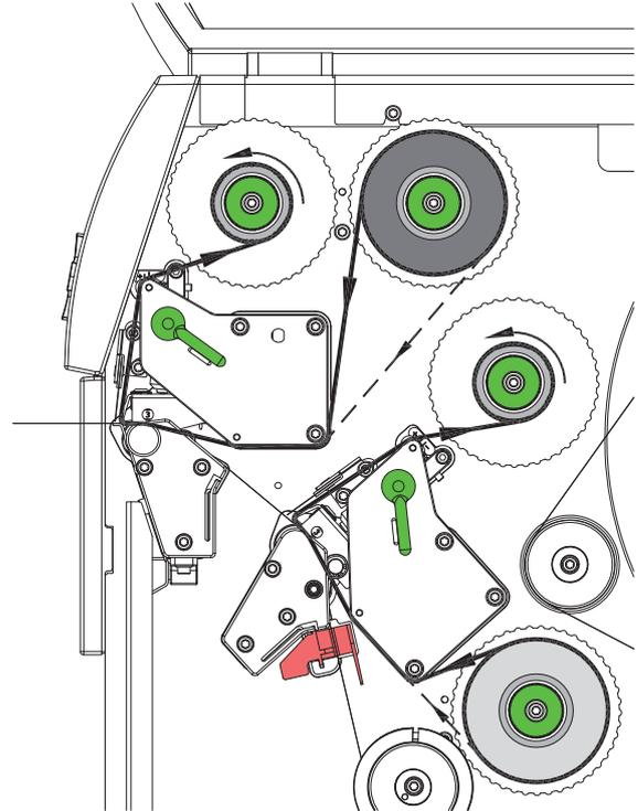
Fig. 15 Transfer ribbon feed path
