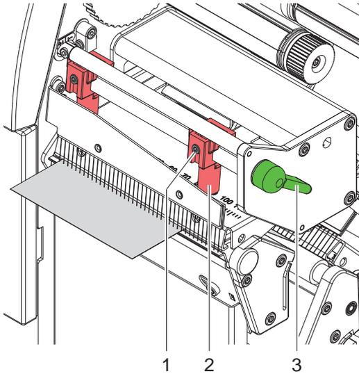
Fig. 12 Setting the upper head locking system
