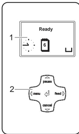
The control panel consists of a graphic display (1) and the navigator pad (2) with five integrated keys.
