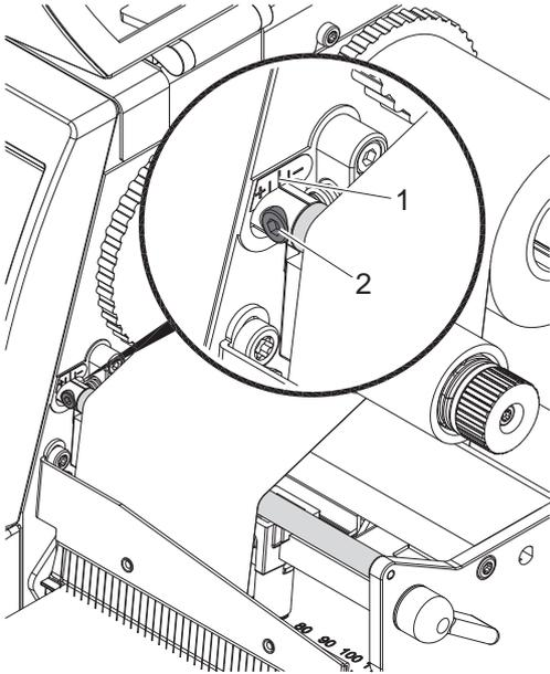
Fig. 16 Setting the upper ribbon feed path
