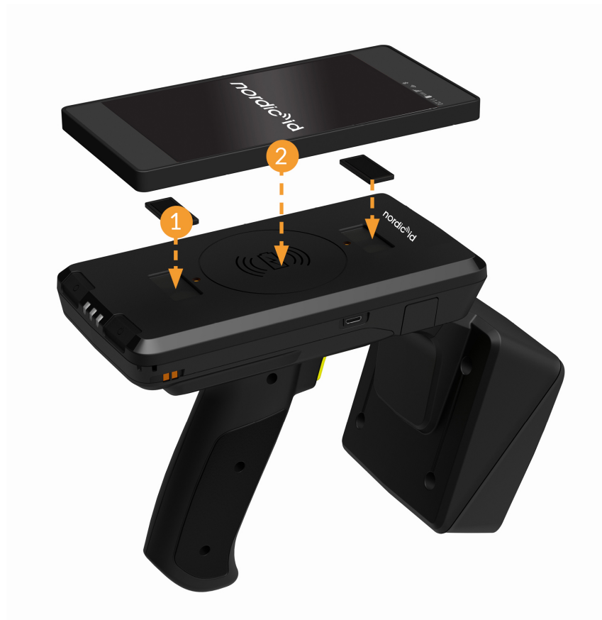
Picture 10 Nordic ID EXA51e fastening with magnets
