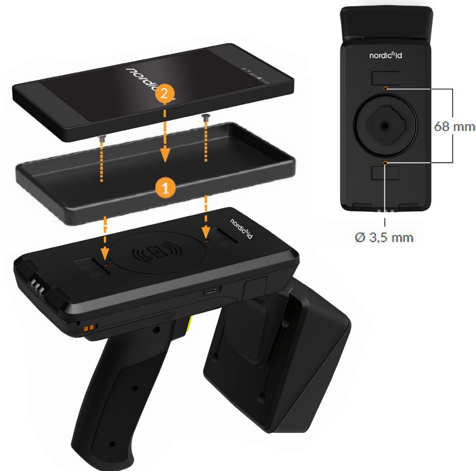
Picture 11 Nordic ID EXA51e fastening with screws
