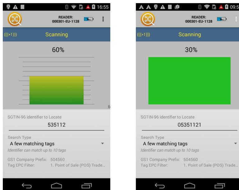
**FIGURE 3:** Bar Graph display mode (left) and Block display mode (right)
