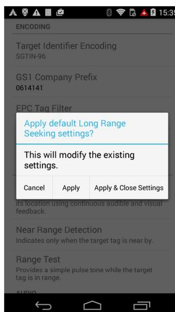
**FIGURE 8:** Resetting to the Long Range Seeking configuration
