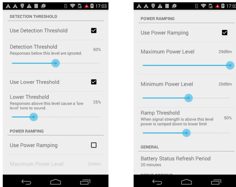
**FIGURE 10:** Settings for Detection Threshold (left) and Power Ramping (right)
