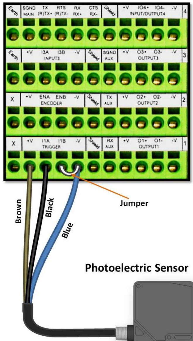
Figure 25: Photoelectric Sensor Wiring (PNP Output)
