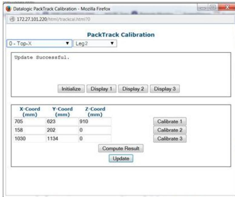
37. Close the **PackTrack Calibration Wizard** window. **PackTrack Calibration Coefficients** have been populated on the Scanner Mounting window.
