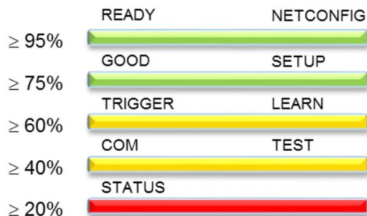
Figure 39: X-Press LED test mode read rate percentages
