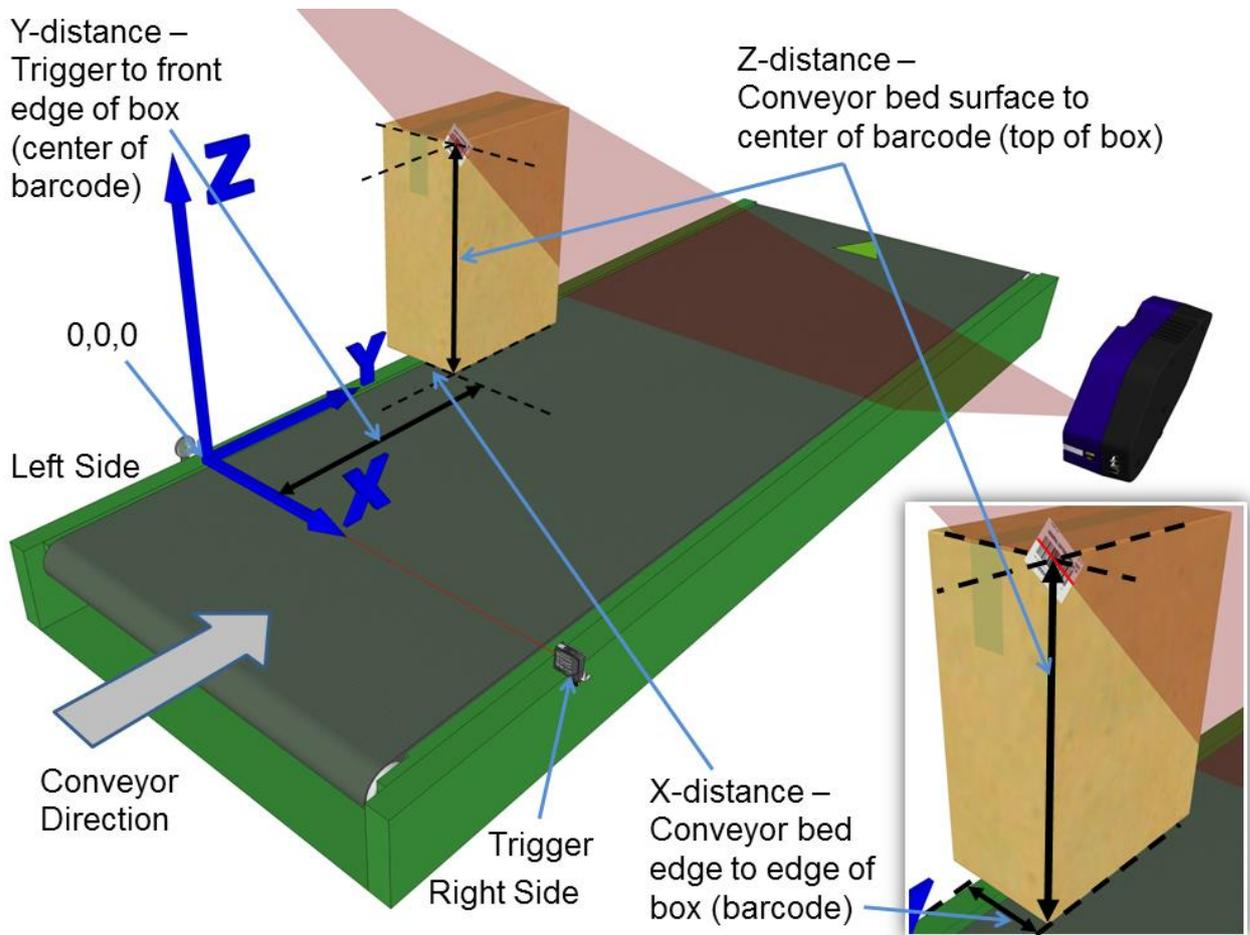
Figure 52: Side-read 2<sup>nd</sup> barcode placement
