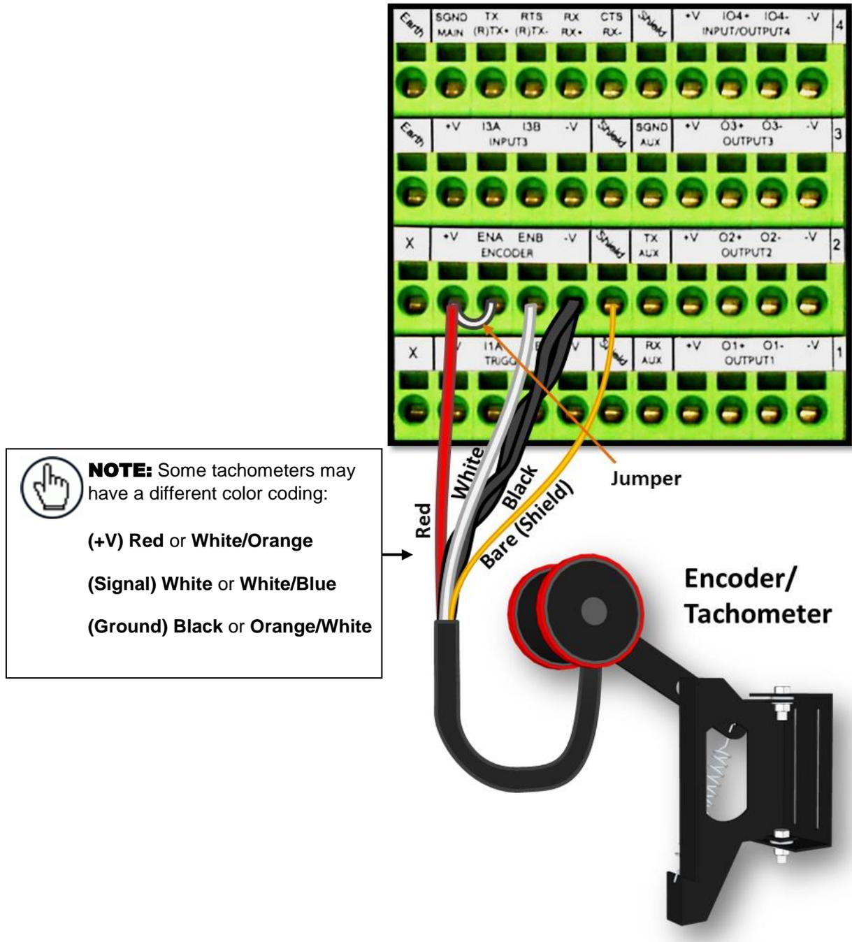
Figure 26: OEK-2 Encoder/Tachometer Wiring (NPN Output)
