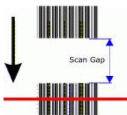
**Code Different When Code Position Gap Is Greater Than** This parameter is available only when the **Code Combination** parameter is set to **Code Collection**. If the position gap between two consecutive codes read (by the Master or Stand Alone scanner) on the same scan line is greater than the defined gap number, the codes will be considered as different.
