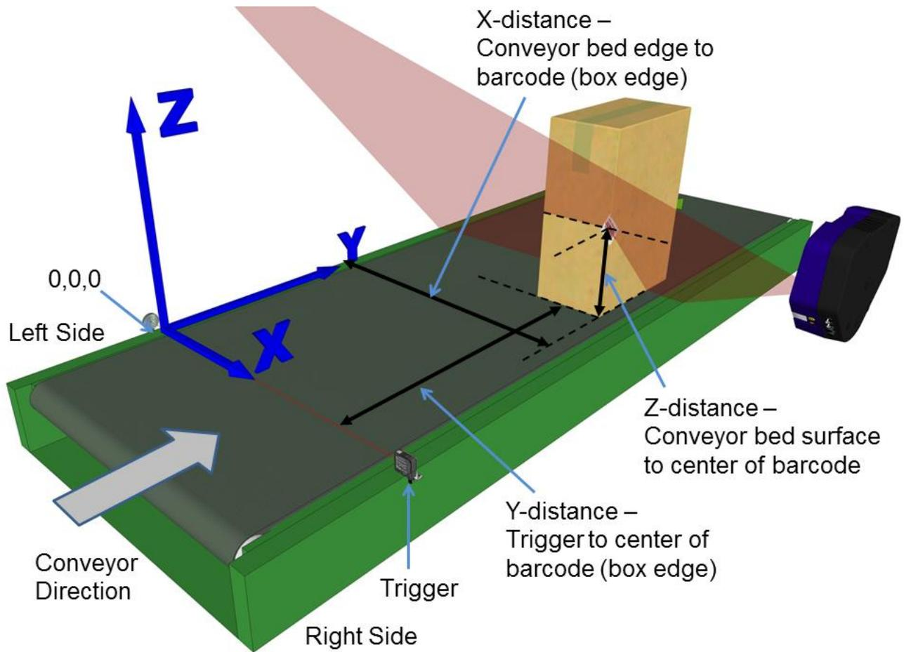
Figure 53: Side-read 3<sup>rd</sup> barcode placement
