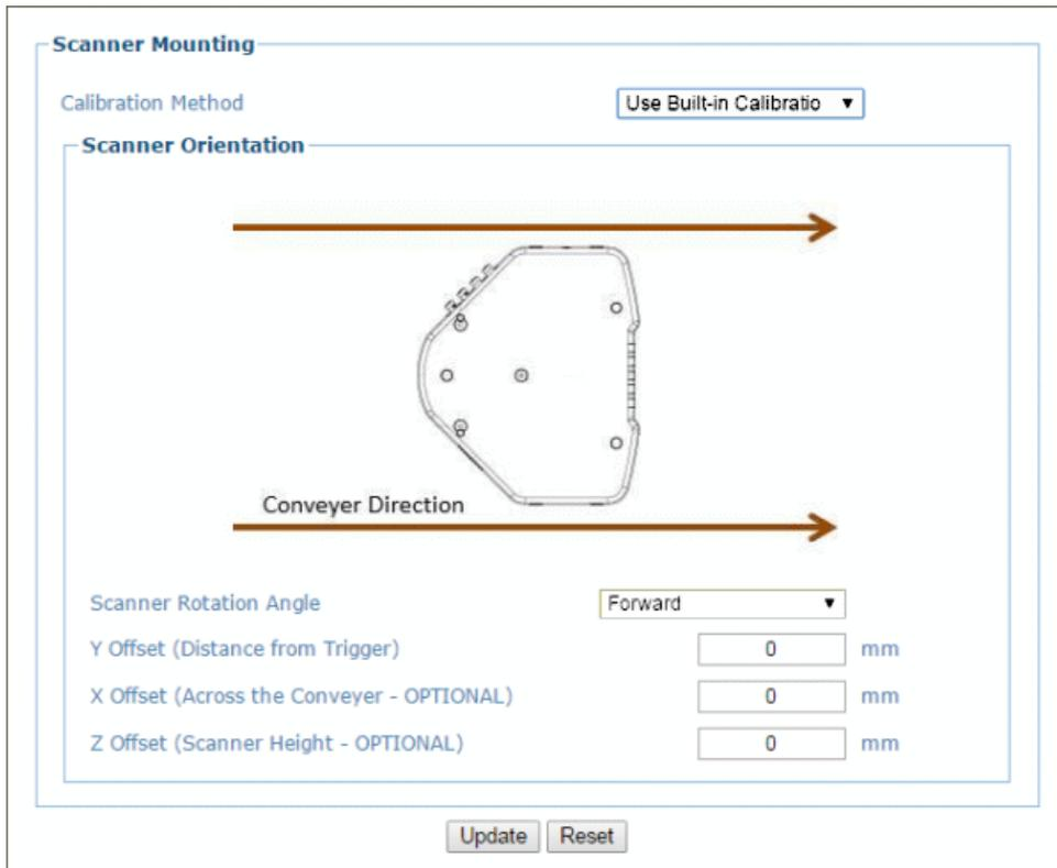
3. Select the scanners orientation to the conveyer from the **Scanner Rotation Angle** drop-down list. Selections include:
