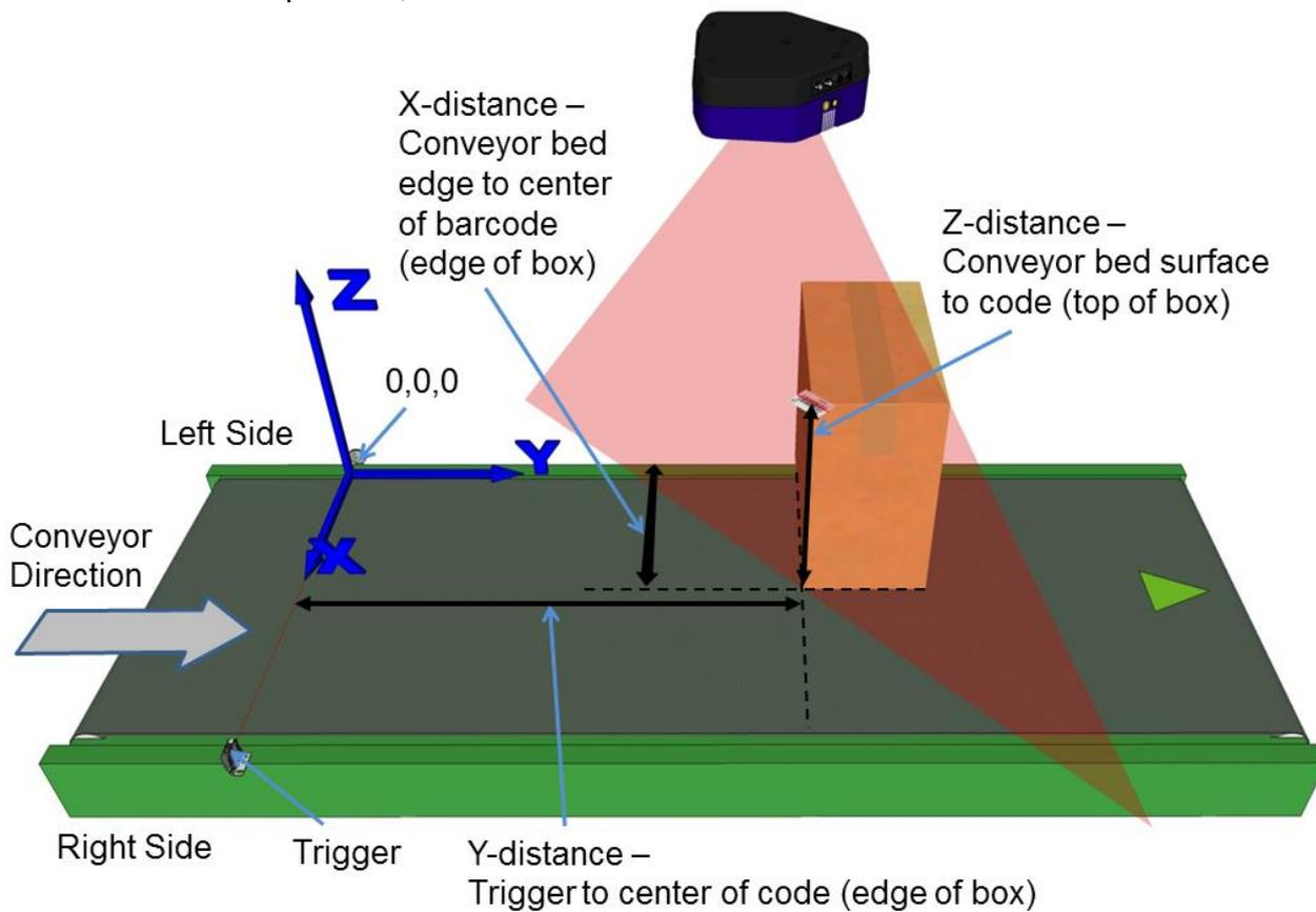
Figure 47: Top-read leg 2- 1<sup>st</sup> barcode placement
