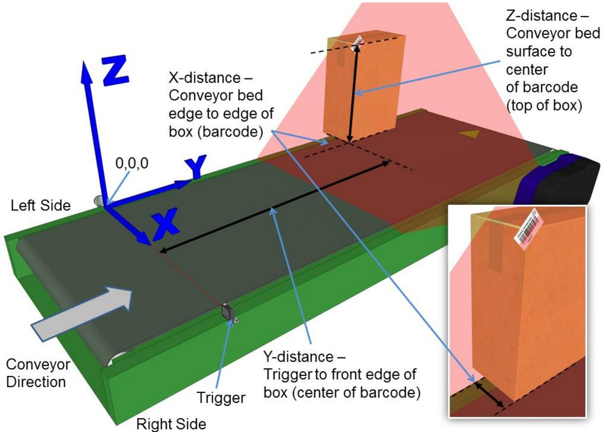
Figure 55: Side-read 2<sup>nd</sup> barcode placement
