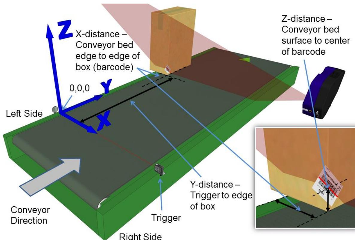
Figure 50: Side-read 1<sup>st</sup> barcode placement
