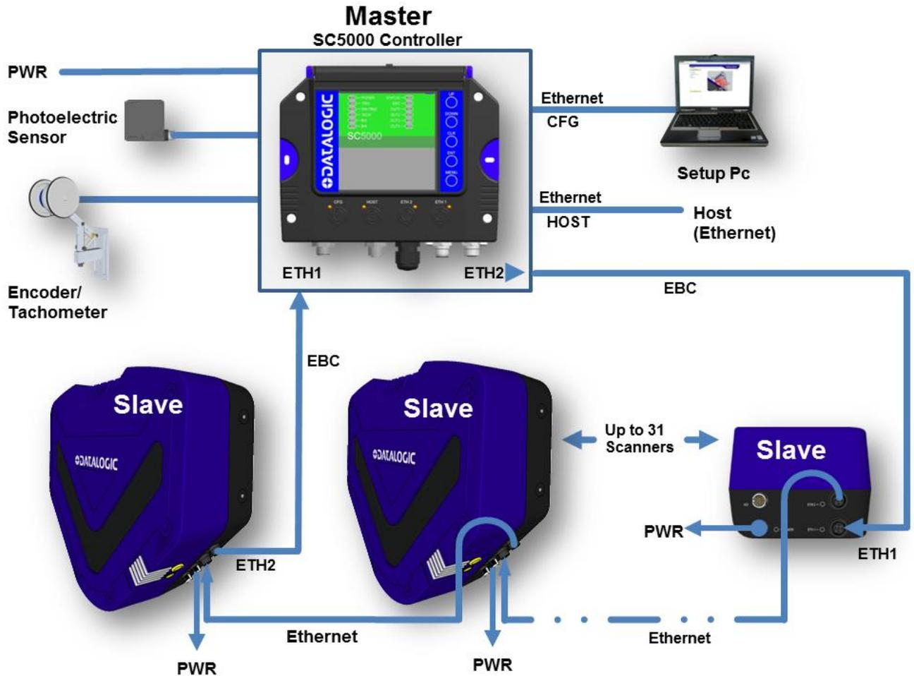
Figure 19: DX8210 Array (Tunnel) with SC5000
