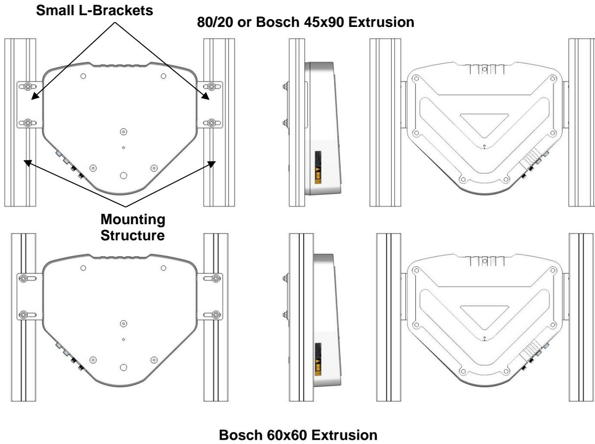
Figure 16: DX8210 Small L-Brackets Mounting Options (93ACC0079)
