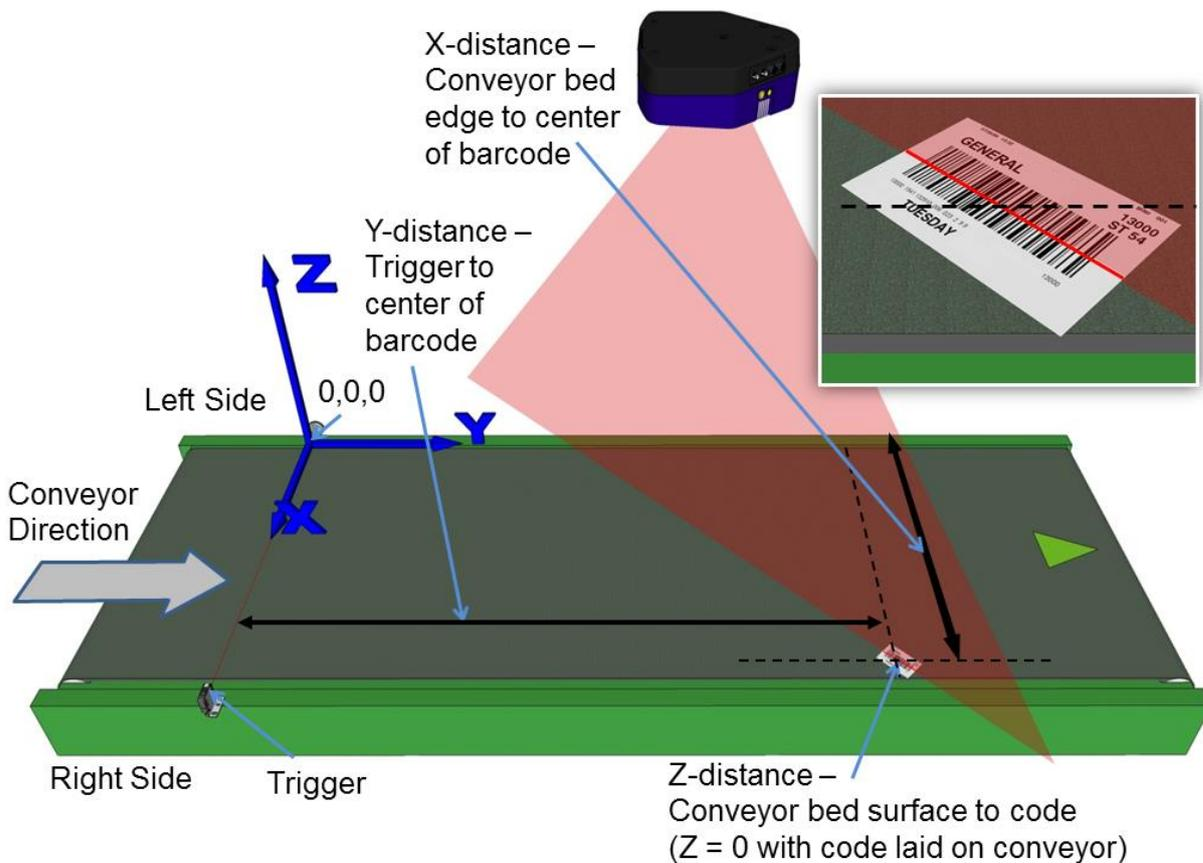
Figure 49: Top-read leg 2- 3<sup>rd</sup> barcode placement
