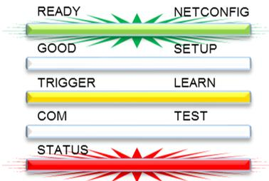
**STATUS/READY + TRIGGER = Motor Failure**
