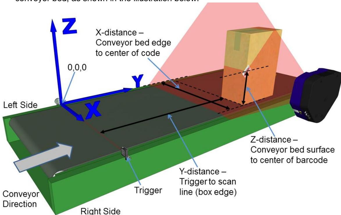
Figure 56: Side-read 3<sup>rd</sup> barcode placement
