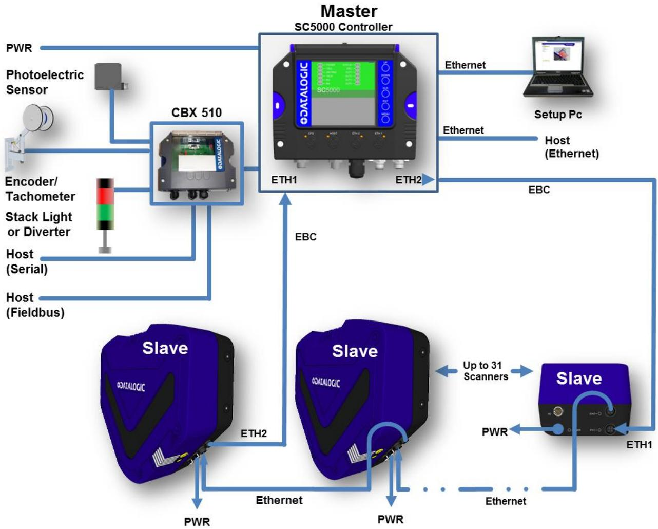
Figure 20: DX8210 Array (Tunnel) to SC5000 (alternate with CBX)
