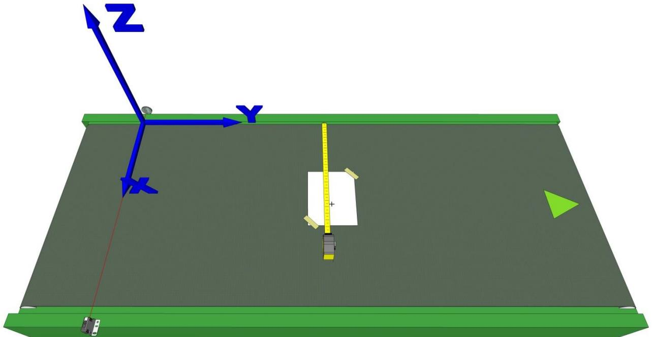
Figure 60: Measuring the X Offset
