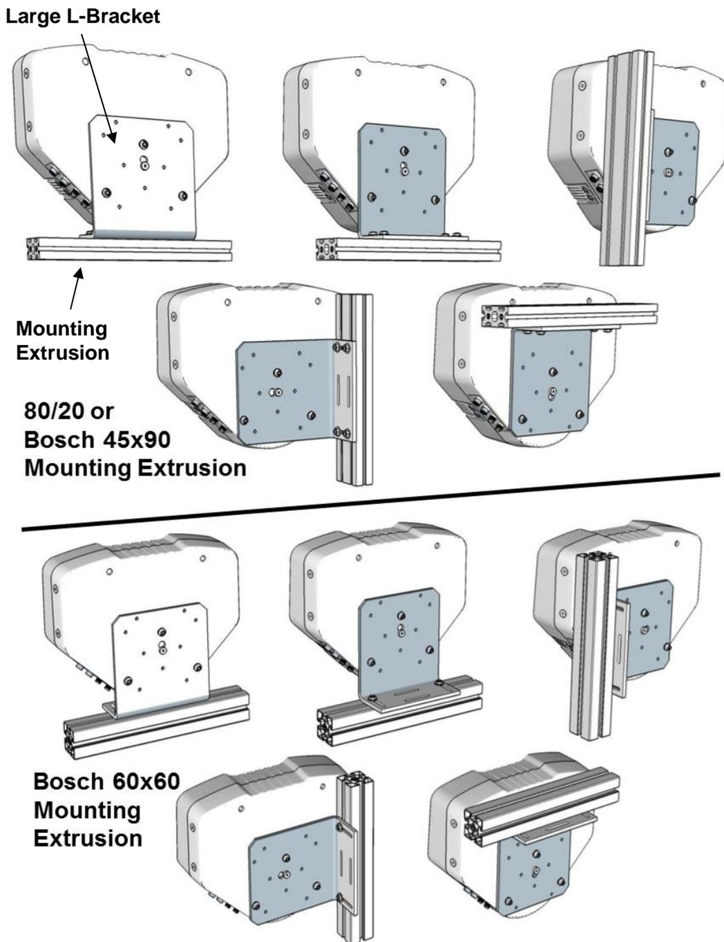
Figure 13: DX8210 Large L-Bracket Mounting Options (93ACC0151, Included with Reader)
