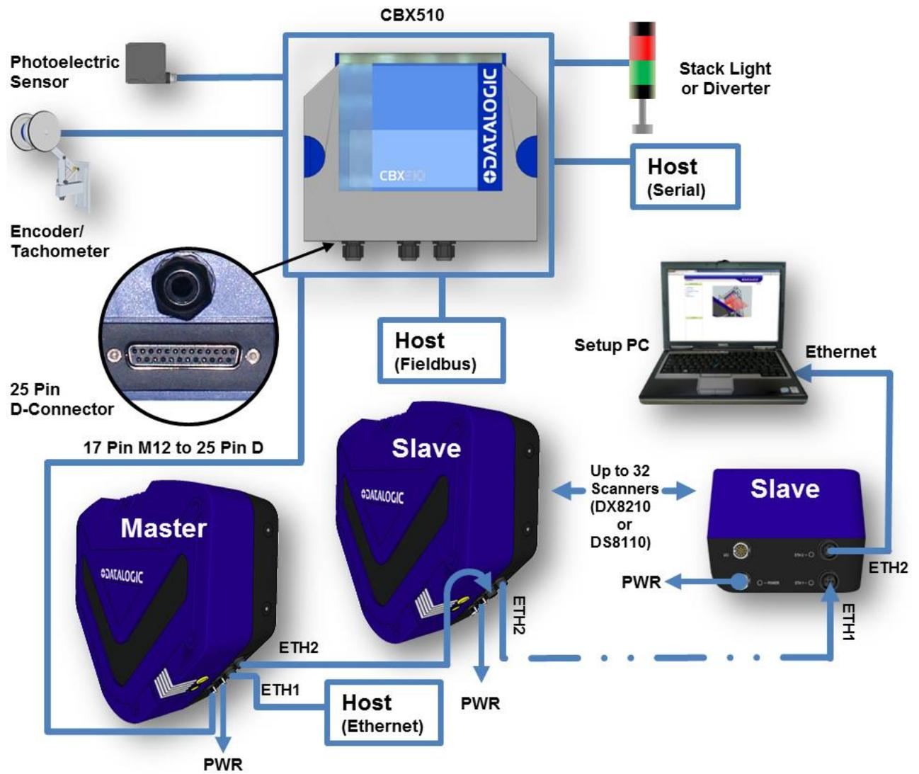
Figure 18: DX8210 Array (Tunnel) to CBX510
