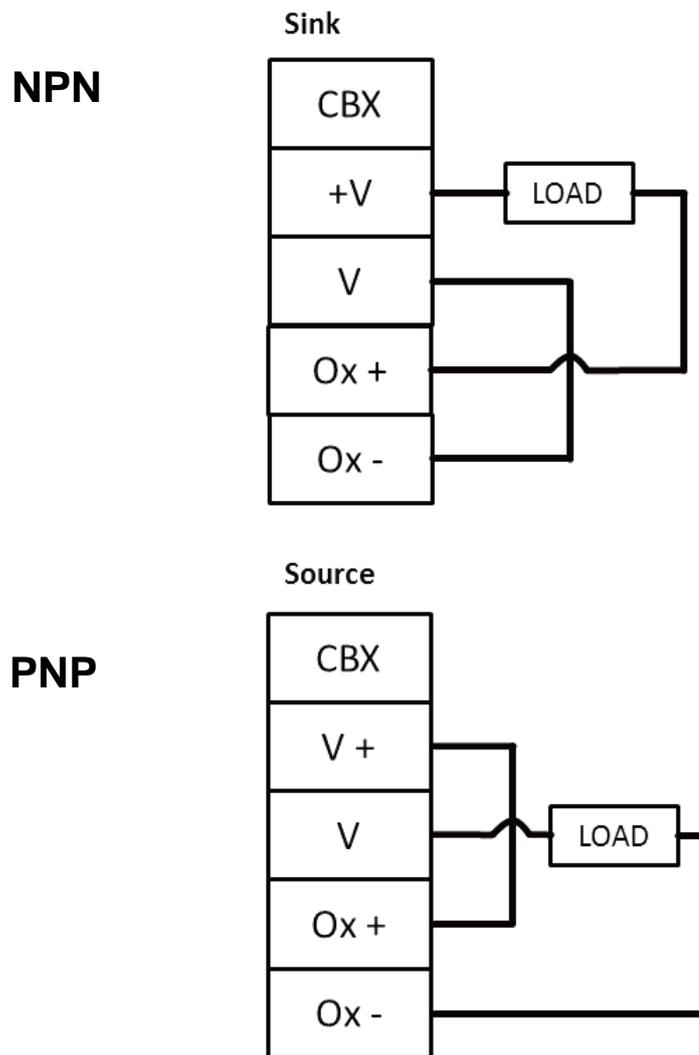
Figure 32: Powered Outputs
