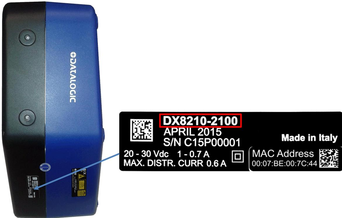
Figure 74 – Identifying the scanner model
