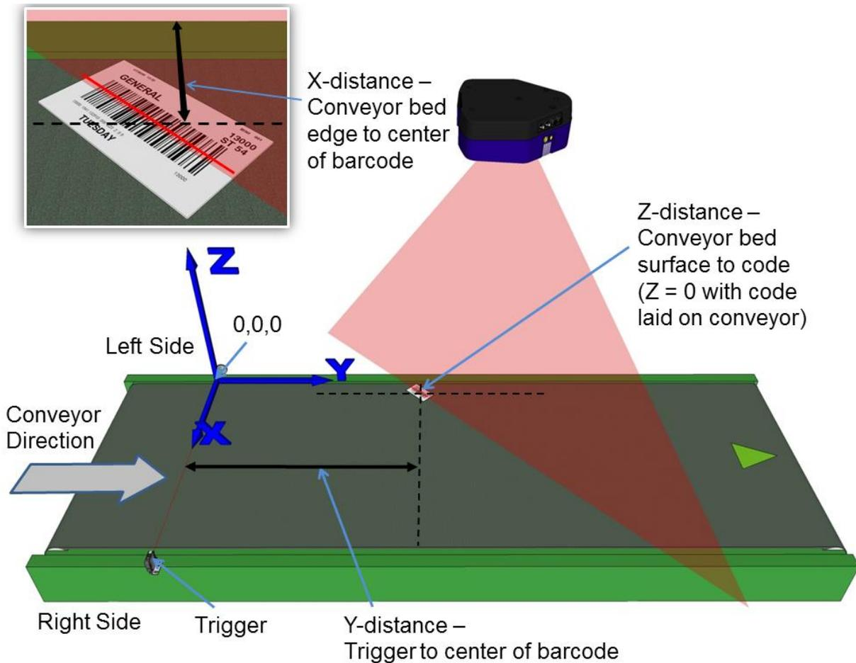
Figure 48: Top-read leg 2- 2<sup>nd</sup> barcode placement
