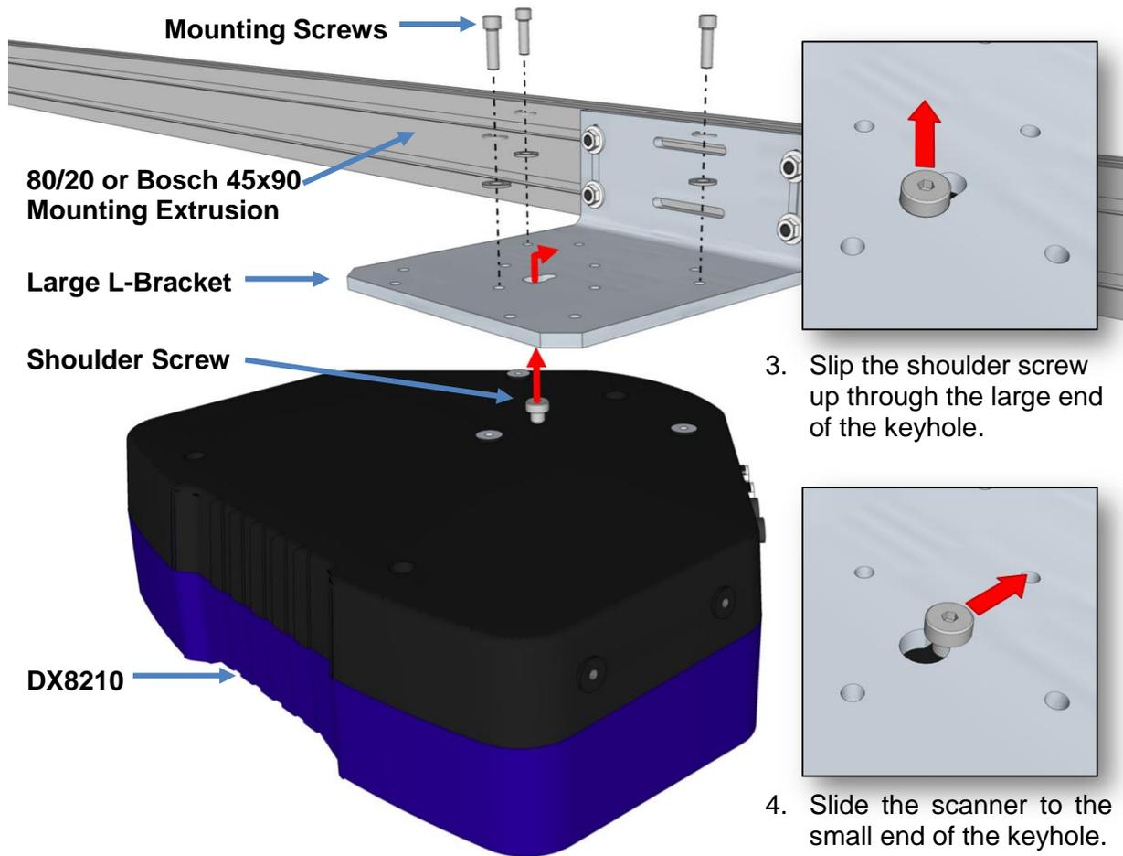
Figure 15: Keyhole mounting with large L-Bracket (80/20 or Bosch 45x90 Mounting Extrusion)
