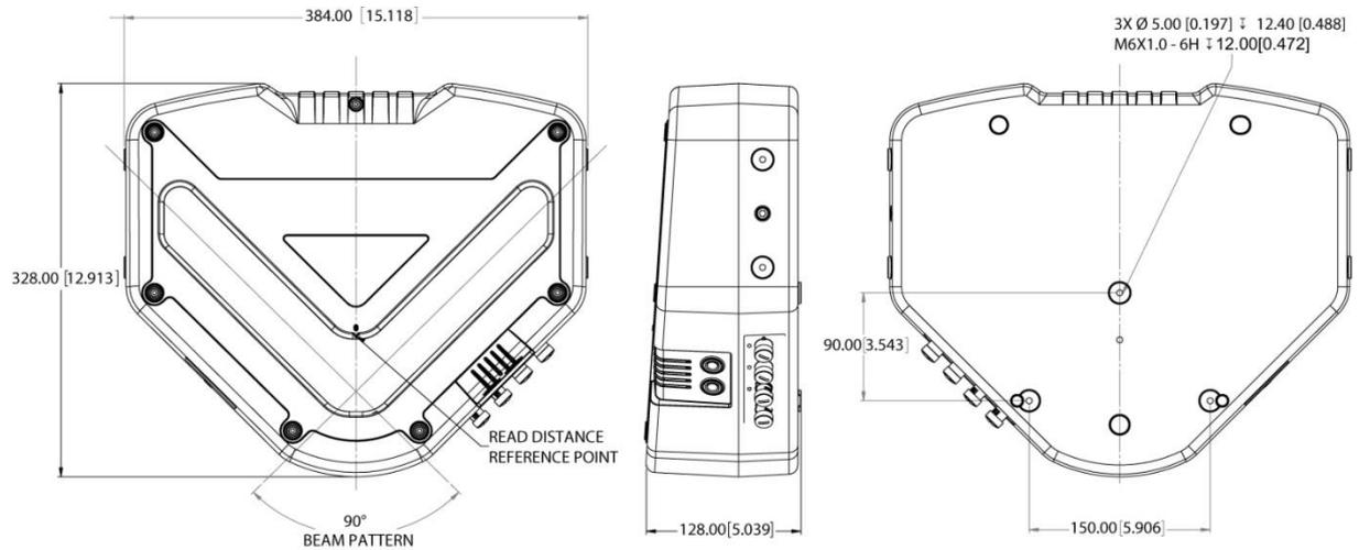
Figure 12: DX8210 Overall Dimensions
