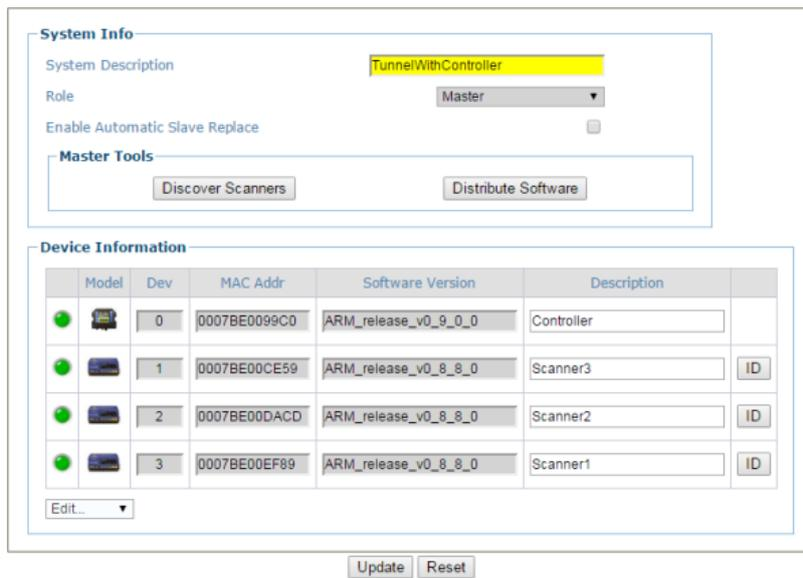
11. If Master is selected, the system is poled, and the other scanners are added to the Device information list. The SC5000 Controller always serves as the Master when used.
