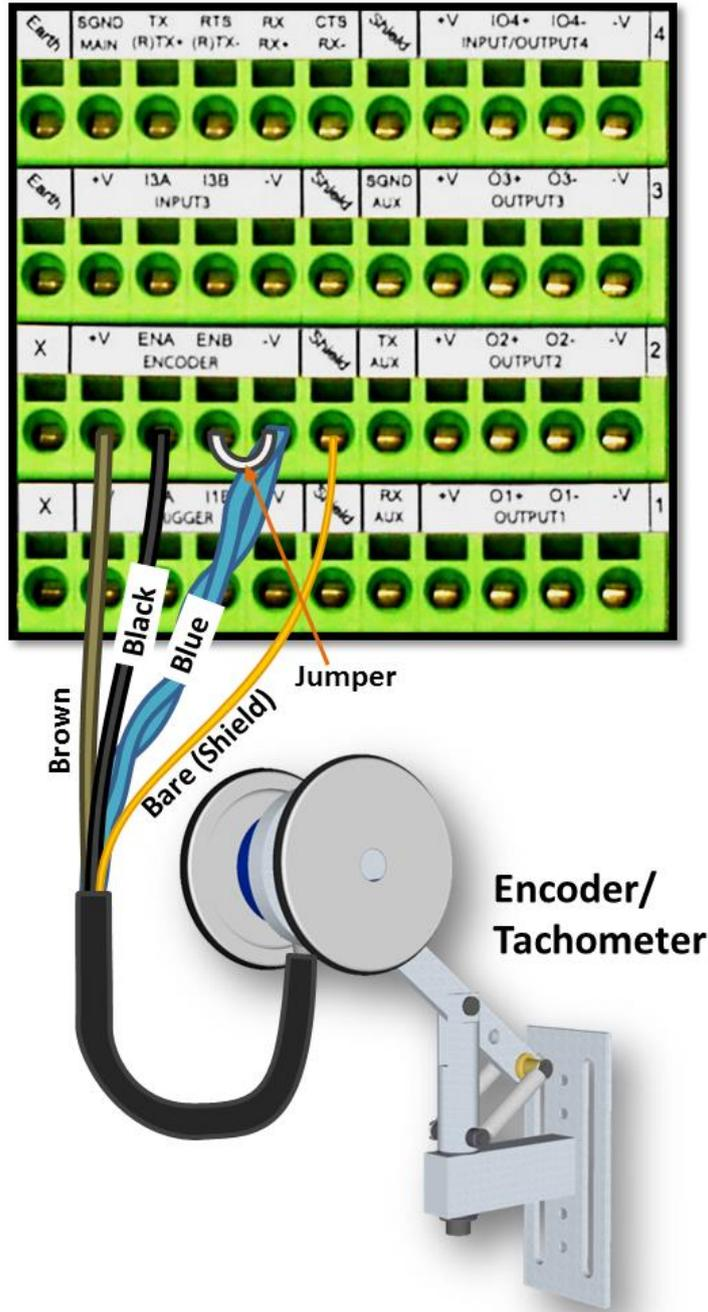
Figure 29: OEK-4 (95B082050) Encoder/Tachometer Wiring (PNP Output)
