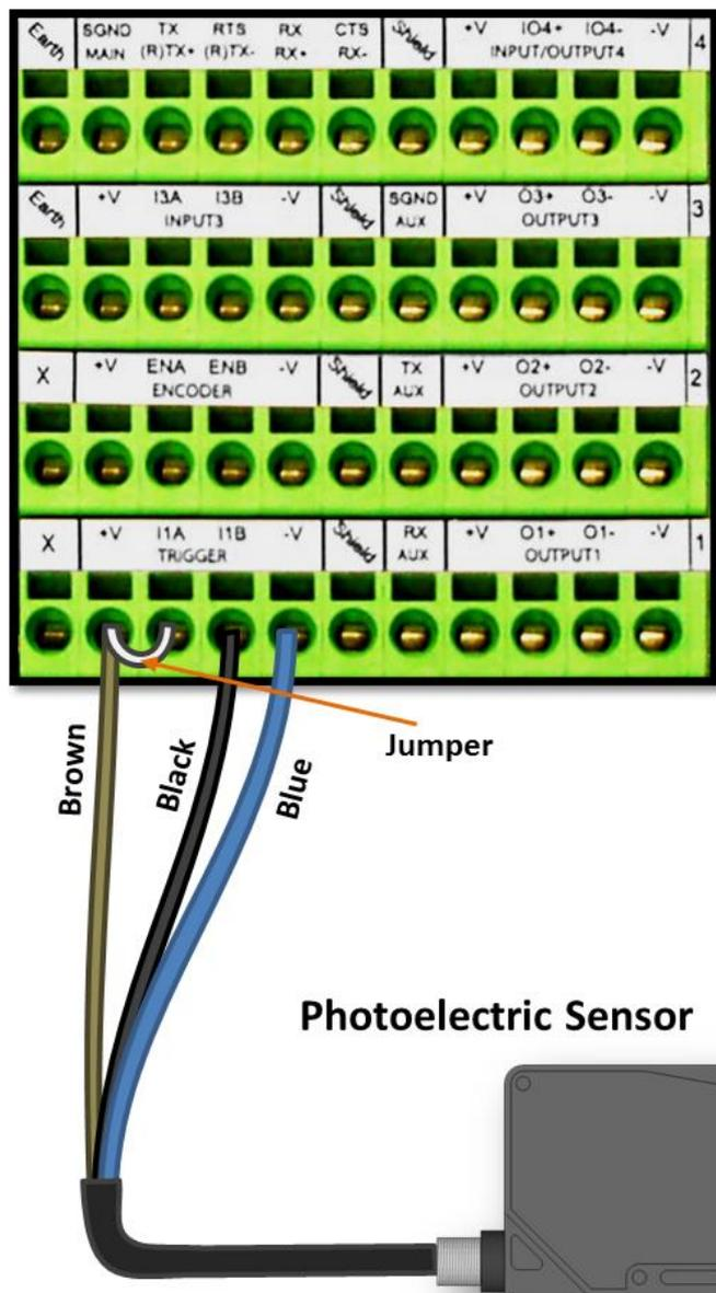
Figure 24: Photoelectric Sensor Wiring (NPN Output)
