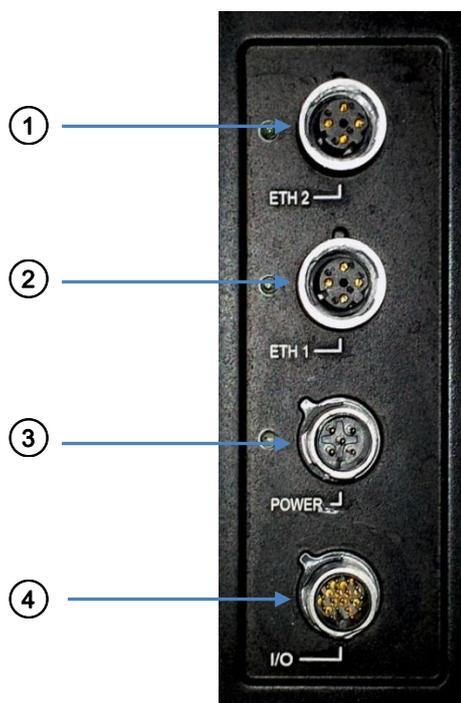
Figure 21: DX8210 Connector Panel
