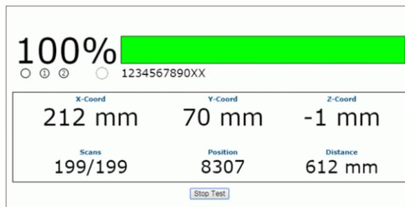
4. Physically measure the X (from left edge), Y (From PS), and Z (code height) coordinates of your test barcode, and compare your measured results to the Read Test results. Your measured results and those displayed should be close (within a few millimeters) but do not need to be exact.
