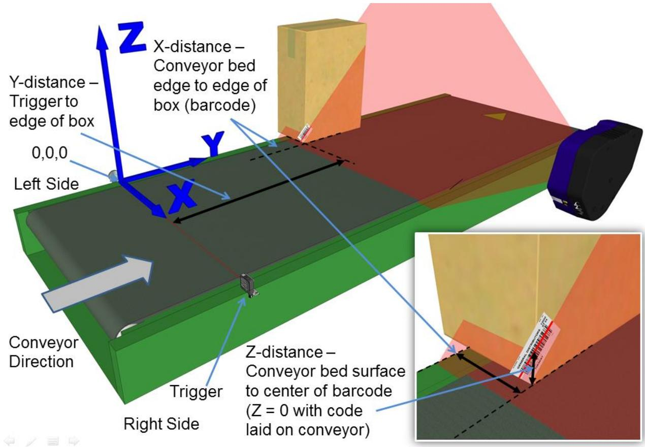
Figure 54: Side-read 1<sup>st</sup> barcode placement
