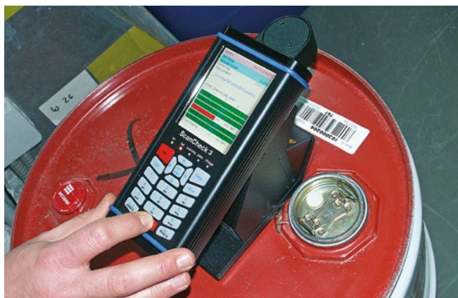
Verifying barcodes on metal barrels
