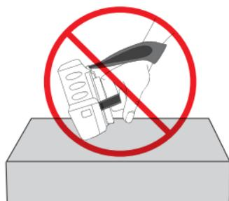
Do not tilt the printer forward or backwards while printing.
