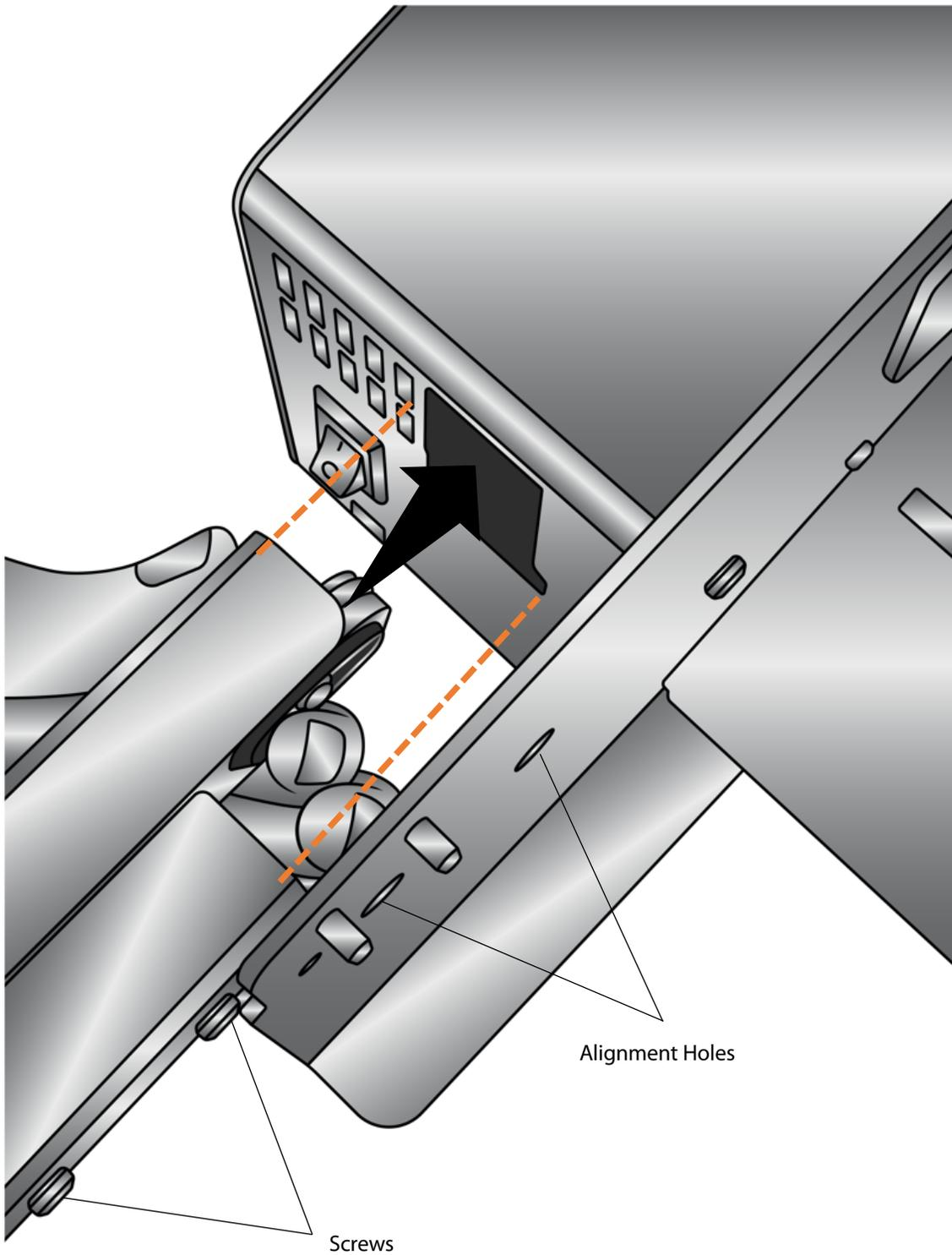
4. Align the screws on the side of the arm with the holes in the applicator frame.
