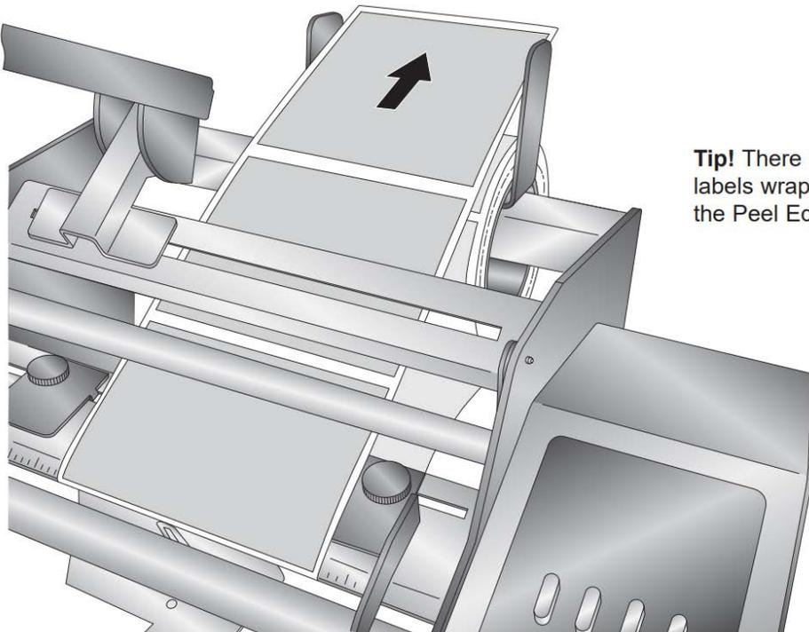
**Tip!** There must be no labels wrapped around the Peel Edge.
