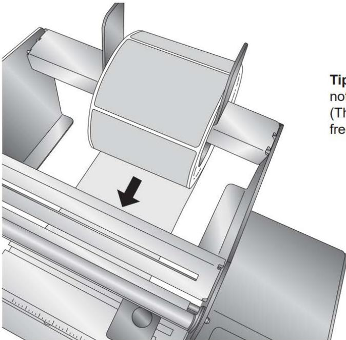
**Tip!** Roll Guide Uprights must not pinch the label stock roll. (The label stock roll must have free-play between guides.)
