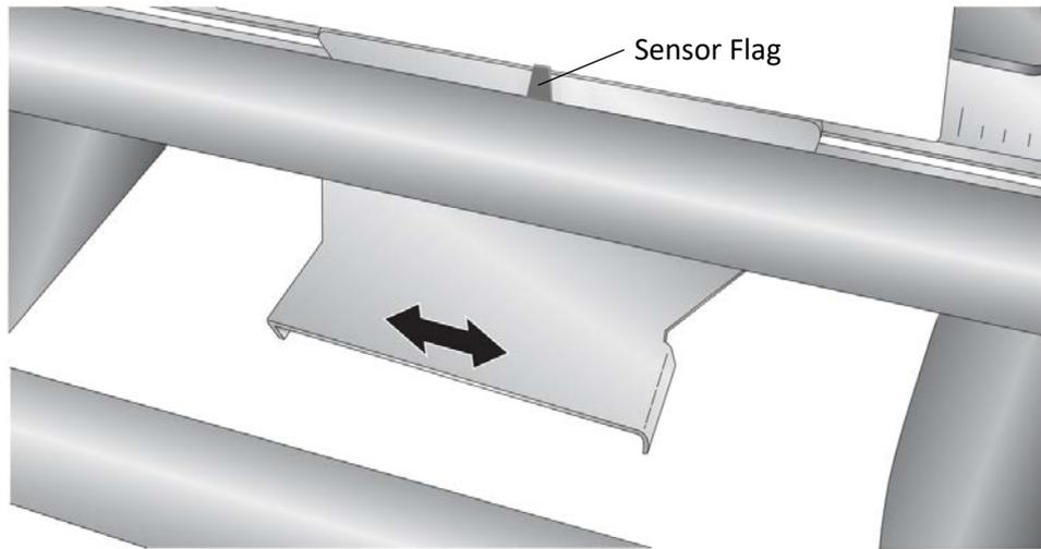
12. Push the liner idler roller into the clamped position.
