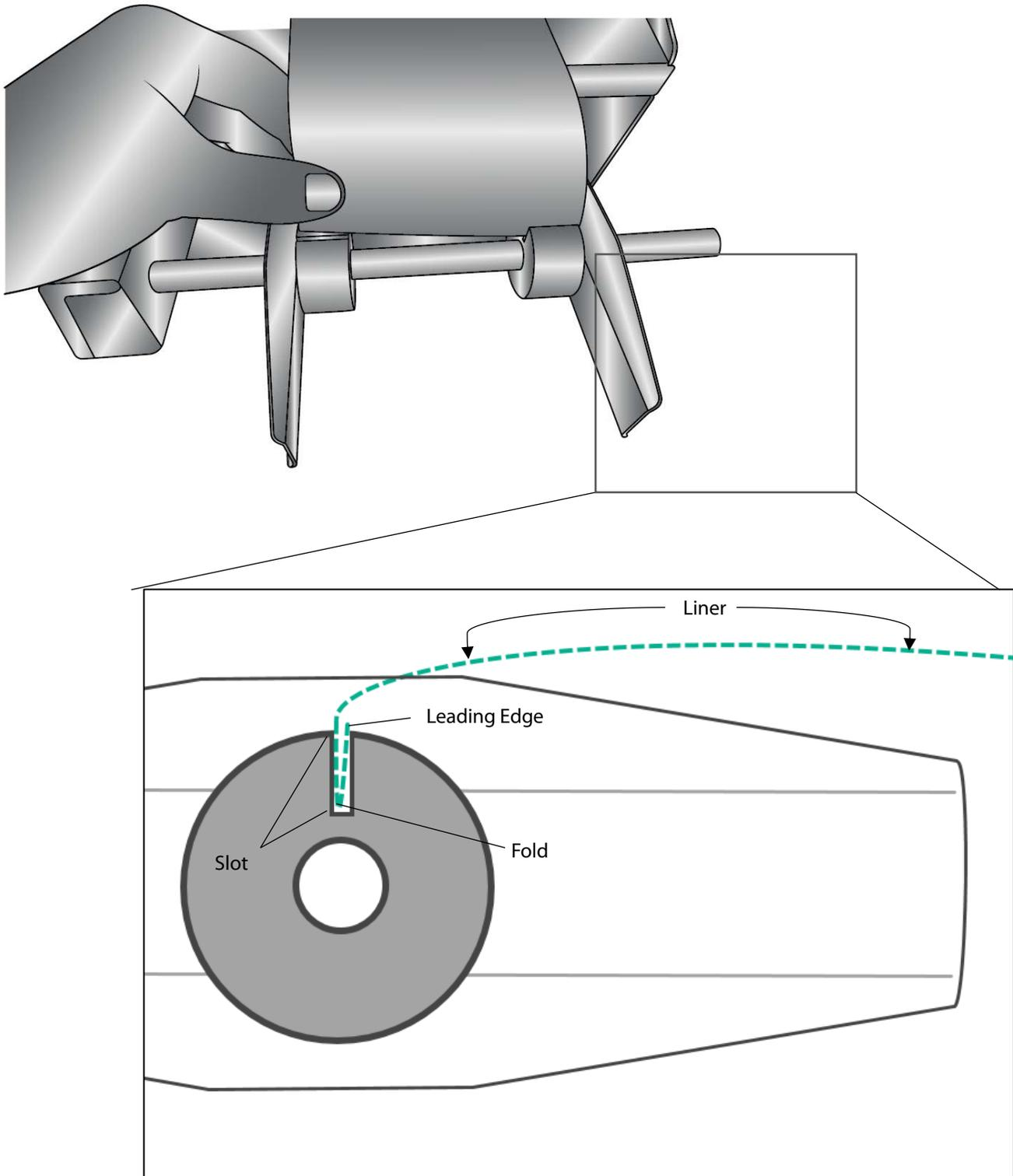
**Tip:** If the liner is slippery and doesn't fold well or stay in the slot, you can tape the liner to the guides to keep it in place. Use low tack tape that has a long cure period such as blue painters tape. You may also use the applicator without using the liner rewinder by removing the liner guides and letting the liner fall over the shaft onto the floor.
