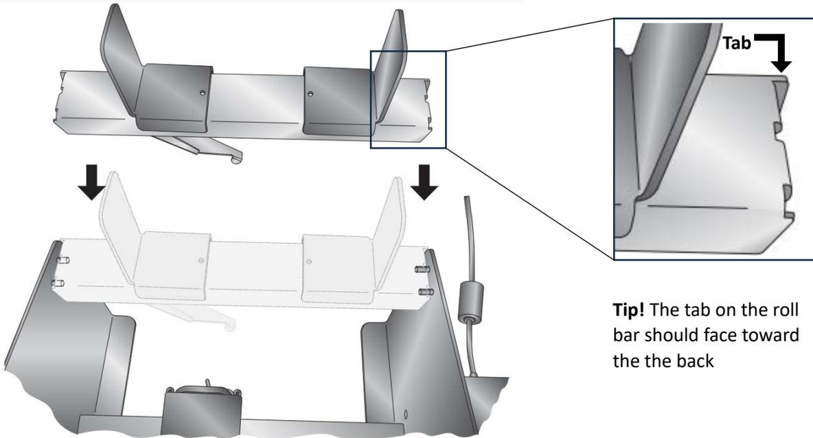
**Tip!** The tab on the roll bar should face toward the the back
