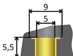
Ideally the tag is placed on large even metal surface with direct metal contact underneath the whole tag. If placement to edge is needed follow below guidance on positioning and leave metal on the left side for the best performance. Tag polarization is along the longest dimension.
