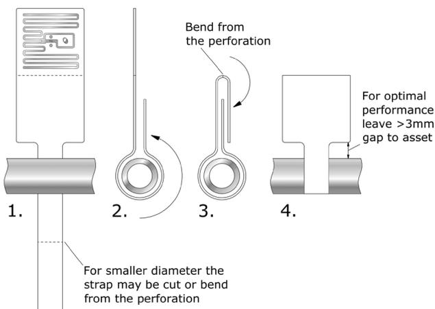
Ideal installation conditions are +20°C (+68°F) / 50% RH. For exceptional conditions, please contact Confidex. Bond strength can be improved with firm application pressure.
