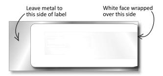
Minimum bending diameter of the Confidex Silverline Classic  $\Pi^{\text{TM}}$  is 100mm. For optimal performance please bend the label in the orientation shown below.
