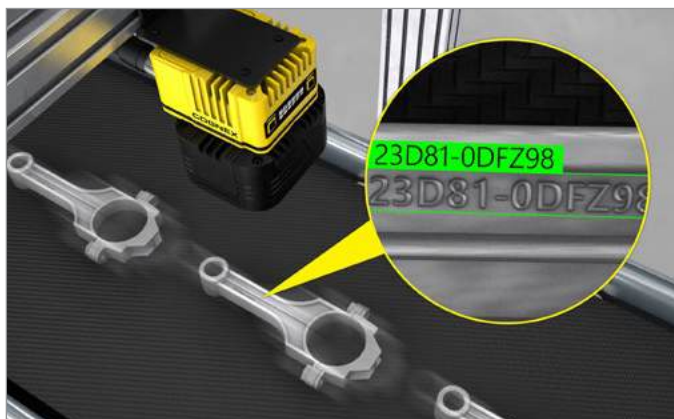
Automotive: Decipher hard-to-read text etched on metallic surfaces
