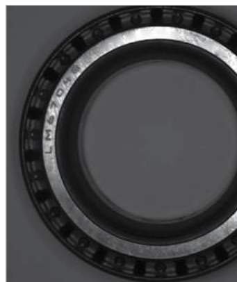
Without HDR: Embedded parts are unclear.
