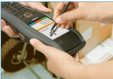
The 8,99 cm transfective colour LCD is produced by CASIO. A user friendly data input and signature capturing method can be done with the touch pen and scratch-resistant touch screen of the device. No matter if glaring sunlight or night delivery – the graphic display with 240x320 pixels is readable under all light conditions.
