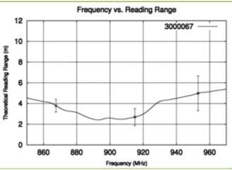
Presented reading ranges are calculated values in non-reflective environment, in where antennas with optimum directivity are used with maximum allowed operating power: EU 865-868 MHz (2W ERP), US 902-928 MHz (4W EIRP), and JPN 952-954MHz (4W EIRP). Variation of 3σ from test batch marked in the picture.
