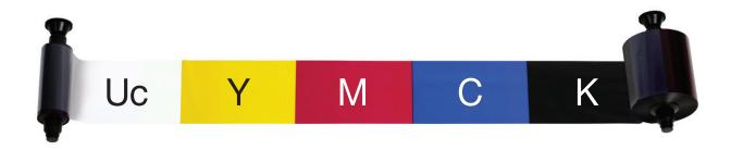
Unichroma<sup>™</sup> is a dry coating (Uc) invented by ITW Imagedata. The special coating is supplied on a color ribbon as a panel that is printed in advance of the following Y, M, C, K panels. The clear, colorless Unichroma<sup>™</sup> coating (Uc) is applied directly to the surface of the card using a normal direct-to-card printer. Then, D2T2 (Dye Diffusion Thermal Transfer) color personalization can continue in the normal way (single or double-sided printing).
