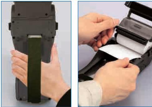
The built-in thermal printer uses a simple one-step paper-loading method. All that is required is to place a paper roll inside the paper roll holder, pull out some paper and then close the cover. This simple method saves time and ensures that the paper is always loaded correctly even when performed in the field.
